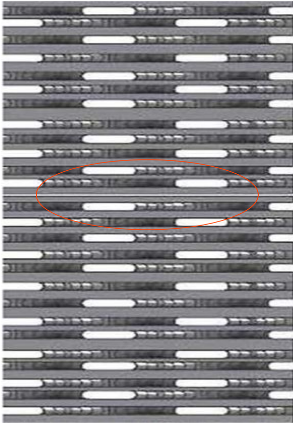
Circle shows two 1/8" (3.2mm) outer high edges forming 1/4" (6.35mm) joint
